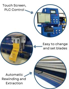
The ULTRA SM 2.0 Multi-Blade Cutting Machine is a cuttingedge solution for manufacturing sheer elegance or zebra shades in high volumes. This state-of-the-art machine is equipped with four cutting heads to simultaneously cut multiple shades at once, ensuring large quantities of fabric can be cut with precision and speed. Using this tool helps to minimize waste and maximize production efficiency.
